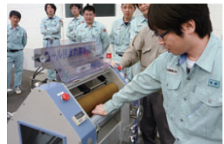
Experience-based training (We are working to prevent accidents through training that simulates occupational accidents caused by being caught in a machine.)
